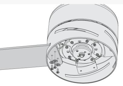
Put the blade washers found in the hardware bag onto the blade screws found in the hardware bag. Then install the blade screws to secure each blade to the fan.
