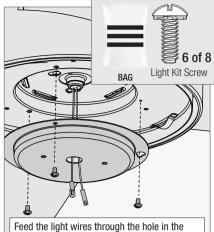
Feed the light wires through the hole in the lower switch housing. Align the lower switch housing screw holes with the bottom of the light kit assembly. Using the three light kit Screws, found in the hardware bag, mount the lower switch housing to the light kit.
